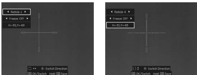
FIGURE 2-9. RETICLE AND BORESIGHTING
