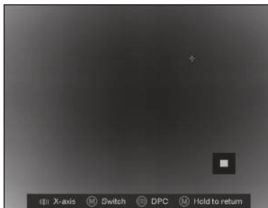
FIGURE 2-6. DEFECTIVE PIXELS CORRECTION
