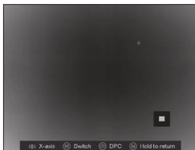
FIGURE 2-6. DEFECTIVE PIXELS CORRECTION
